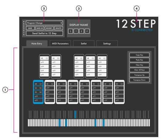
(1) Main Tab Area: Houses the four main editor tabs. See the <u>Note Entry</u>, <u>MIDI Parameters</u>, <u>Setlist</u>, and <u>Settings</u> sections for more detailed information on each tab.
