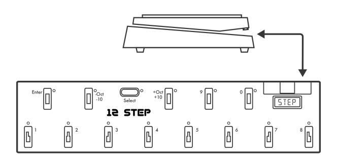
Most standard expression pedals can be directly connected to the 12 Step and used to send MIDI data.
