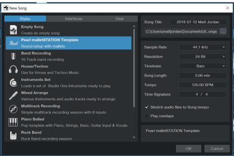
Step 12 – At this point, both *Presonus Studio One 4 Artist* and the *Pearl malletSTATION Sound Set* are installed. Plug your malletSTATION into your computer, and you should then be able to select a track on the left hand side, play the malletSTATION, and hear sounds. Depending on your audio device, you might need to set your latency lower in the Studio One options/preferences to reduce the delay between the time your mallet hits the bars and the time you hear the sound.
