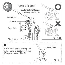
To change to a higher or shorter beater height, loosen the Allen Screw on the Beater Setting Stopper with the provided Multi-Function Drum Key or Allen wench (3mm) then loosen the Key Bolt on the Beater Holder Link (Fig.3). Set the beater to the desired height and re-tighten the Key Bolt. Reset the Beater Setting Stopper flush against the Beater Holder Link per the instructions above.
