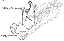
Reattach the Hinge to the Footboard in the position shown with two 3-Piece Screws using the provided Multi-Function Drum Key or Allen wrench (3mm) (Fig.11).
