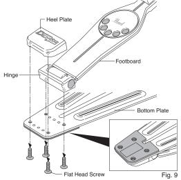
Lift the Footboard and remove the four 3-Piece Screws with the provided Multi-Function Drum Key or Allen wrench (3mm) as shown, and remove the Hinge from the Footboard (Fig. 10).  $\swarrow$
