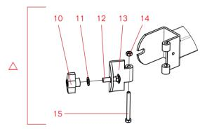
Each connection uses the same clamp and hardware.
